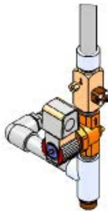
DETERGENT SUPPLY MANIFOLD WITH SOLENOID VALVE AND DEMA INJECTOR
