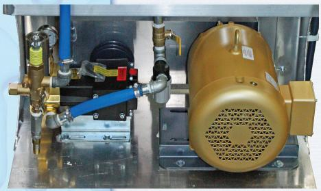
**Electric Motors.** 208/230/460 Volts. 3 Phase, TEFC.
