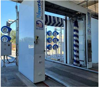
According to Barfield, selecting a new bus wash system was fairly simple. The agency needed a bus wash that could accommodate a 60foot articulated bus, would utilize an updated vacuum rather than a blower system, and could facilitate a two-lane system to increase the number of vehicles washed per day – the agency was looking to run as many as 100 vehicles a night as part of their standard refueling and vaulting process.
